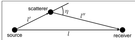
Figure 12: Schematic map view of the single-scattering geometry in our simplified 2D, flat-earth, surface-wave inversion problem. The quantity  $l$  is the horizontal epicentral distance between the source and receiver;  $l'$  and  $l''$  are the lengths of the first and second legs of the detour path, respectively, and the angle  $\eta$  measures the deflection of the wave at the scatterer.
