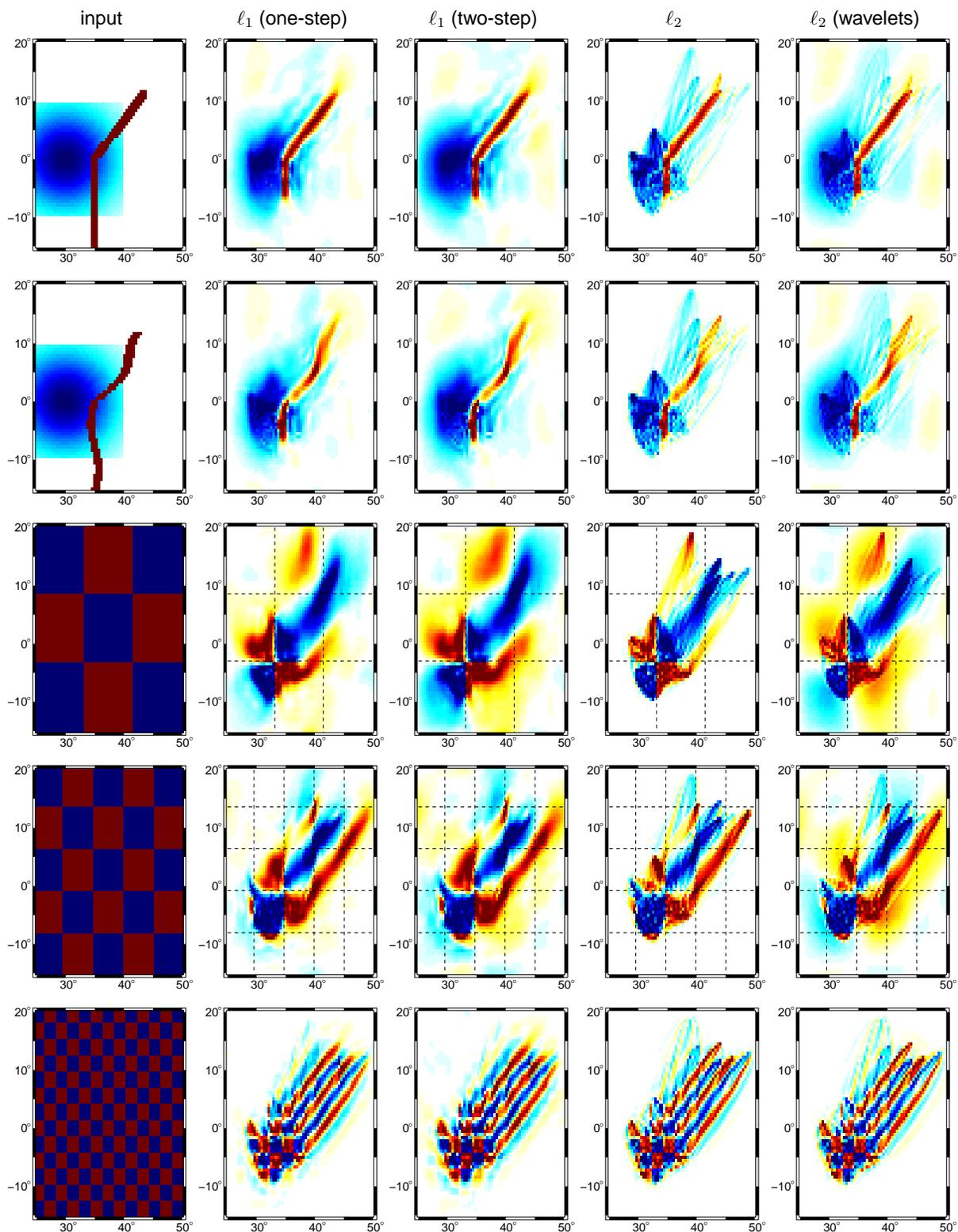
Figure 11: Results of applying different reconstruction techniques to a number of different 2D toy models. From left to right: Original input model;  $\ell_1$  reconstruction (2000 iterations, single-step procedure);  $\ell_1$  reconstruction (1000 + 1000 iterations, two-step procedure);  $\ell_2$  reconstruction (2000 iterations, without wavelets);  $\ell_2$  reconstruction (2000 iterations, with wavelets).
