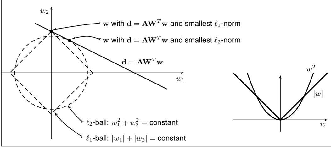
Figure 1: Sparsity,  $\ell_1$  minimization and  $\ell_2$  minimization: Left: Because the  $\ell_1$ -ball has no bulge, the solution with smallest  $\ell_1$ -norm is sparser than the solution with smallest  $\ell_2$ -norm. Right: A  $|w|$  penalization effects small coefficients more and large coefficients less than the (traditional)  $w^2$  penalization.
