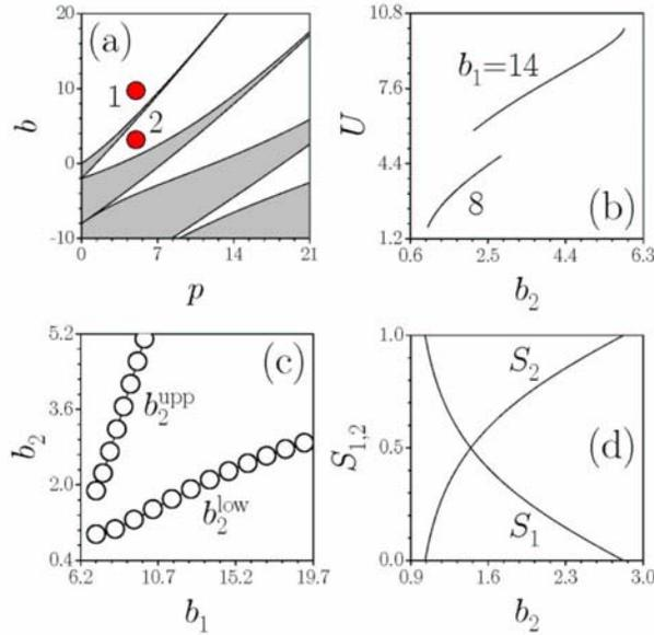
Fig. 1. (a) Schematic representation of the loci of the nonlinear propagation constants of the vector surface soliton components in the band-gap lattice spectrum. (b) Total energy flow vs  $b_2$  at  $p = 5$ . (c) Domain of existence of vector surface solitons at the  $(b_1, b_2)$  plane at  $p = 5$ . (d) Energy sharing between soliton components vs  $b_2$  at  $b_1 = 8$  and  $p = 5$ . Focusing medium. Here and throughout the paper we set  $\Omega = 4$ .
