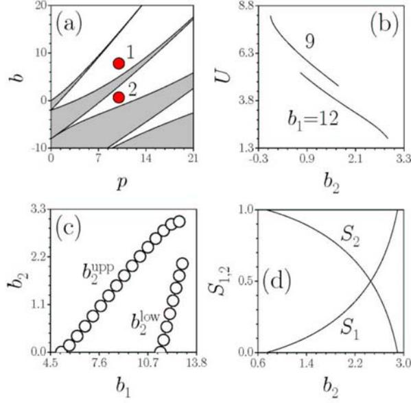
Fig. 3. (a) Representation of the loci of the propagation constants of the vector surface soliton components in the band-gap lattice spectrum. (b) Total energy flow vs  $b_2$  at  $p = 10$ . (c) Domain of existence of vector surface solitons at the  $(b_1, b_2)$  plane at  $p = 10$ . (d) Energy sharing between soliton components vs  $b_2$  at  $b_1 = 12$  and  $p = 10$ . Defocusing medium.
