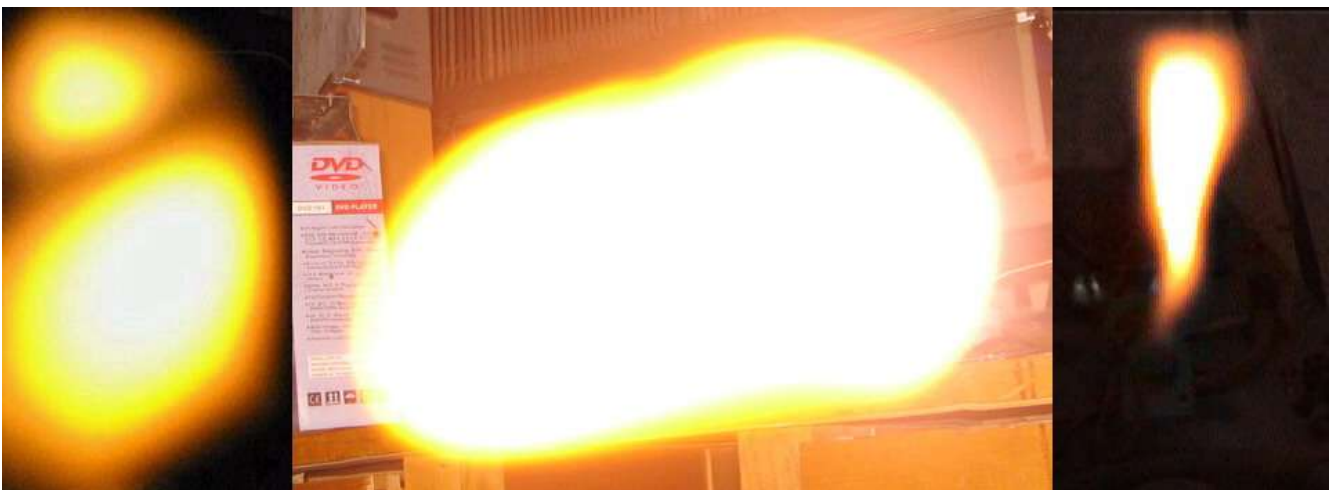
Fig. 4. Different forms of the afterglow of the discharge with carbon electrodes.
