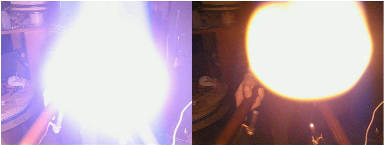
Fig.2. Volumetric discharge with carbon electrodes accompanied with combustion and discharge's afterglow.
