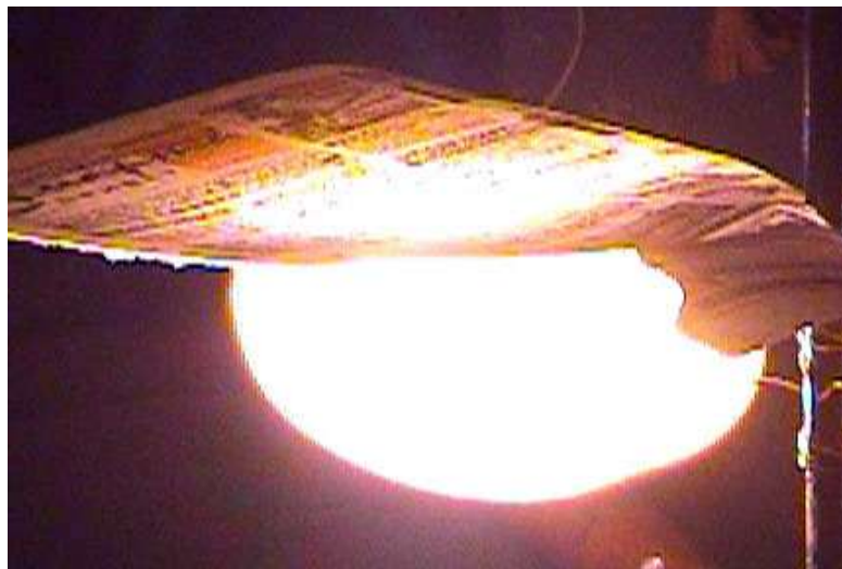
Fig. 6. Heat pulse is insufficient to set fire to a sheet of newsprint.
