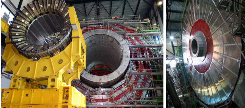
Figure 2. Left: barrel components (front: hadron calorimeter, back: magnet and muon system) of the CMS detector. Right: forward components (muon system) of CMS.
