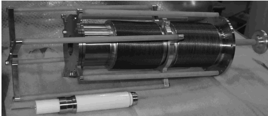
Fig. 4. Bellows system for position control of charger electrode, before attachment to HV test system central volume. The charger electrode protrudes from the right end. The ceramic feedthrough used to bring the initial HV potential into the LHe volume can be seen in the foreground before being welded into place in the small hole in the left end-cap of the bellows assembly.
