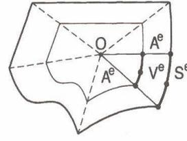
**Fig. (1b) Scaled Boundary (section).**
