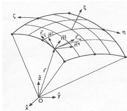
**Fig.(2a). The Scaled boundary transformation of the geometry of the surface finite-element.**
