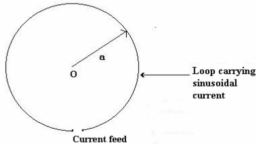
**Figure (3) . A circular loop of radius 'a' carrying a sinusoidal current distribution**
