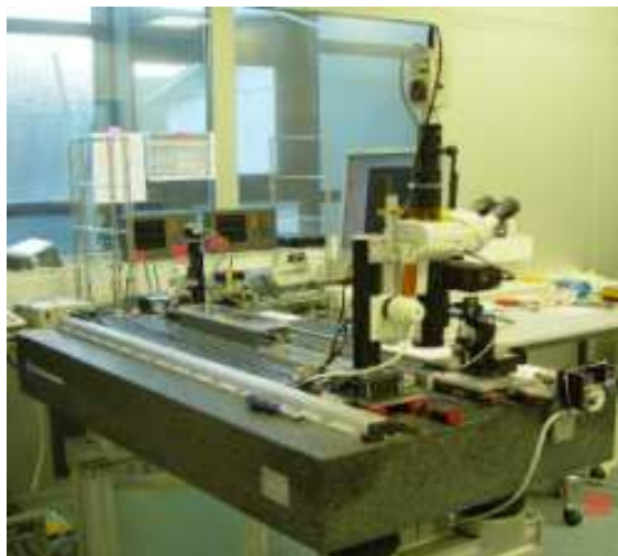
Fig. 5. Wuppertal loading machine with granite table and microscope positioning system
