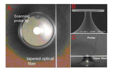
FIG. 1: Optical micrographs of the experiment. Panel A: top view of toroid microcavity coupled to a tapered optical fiber and contacted from the top by a scanning probe tip. Panel B: Scanning electron micrograph (SEM) of the toroid microcavity used to obtain the imaging results shown in Fig. 3. Panel C: side view of a toroid cavity contacted with a scanning probe tip from the top, and with the tapered optical fiber coupled evanescently via the side.
