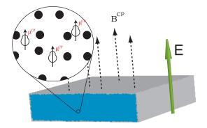
FIG. 1: Scheme of searching for EDM of electron with diatomic radicals embedded in a matrix of rare-gas atoms. A polarizing electric field E is applied to the matrix. As a result, molecular CP-violating magnetic moments  $\mu^{\rm CP}$  become oriented and generate ultraweak magnetic field  $B^{\rm CP}$ . By measuring  $B^{\rm CP}$  one places constraints on eEDM.
