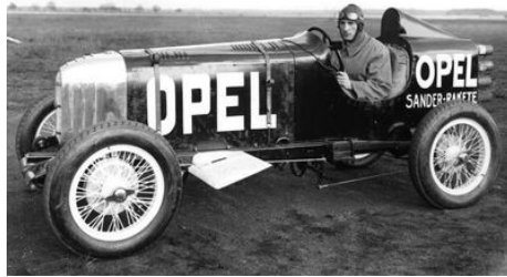
Figure 1: Opel's 1928 experimental rocket car, the RAK 1, with side-wings.
