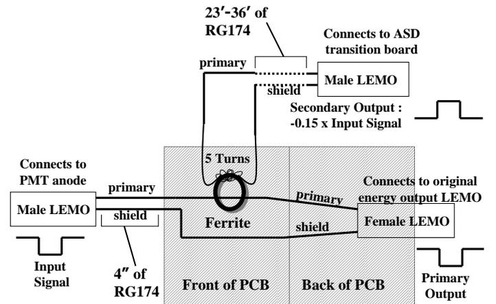
Fig. 2. An electronics schematic for the “splitter” printed circuit board (PCB) used in the CEM timing measurement. Note that RG174 refers to the coaxial cable used in the system, and that the primary output is used for the energy measurement while the secondary output is used for the timing measurement and is the input to the transition boards.
