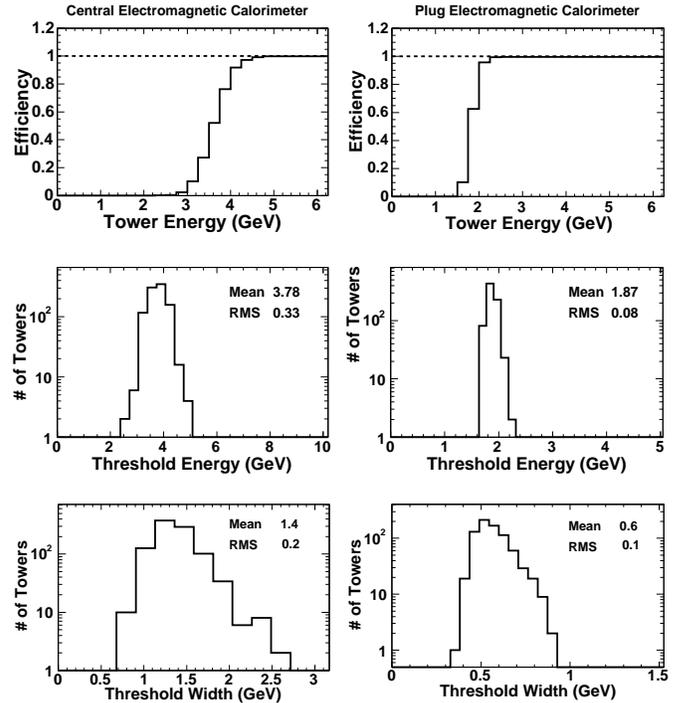
Fig. 4. The EMTiming system response as a function of the energy deposited in the EM calorimeter for a sample of hadrons from jets measured in the detector. The top plots show the efficiency (the fraction of events with a time recorded in the TDC to all events) as a function of the energy for the CEM and PEM, and includes all channels. The bottom two rows show histograms of the energy threshold and threshold width of the individual channels and indicate the uniformity of the system.
