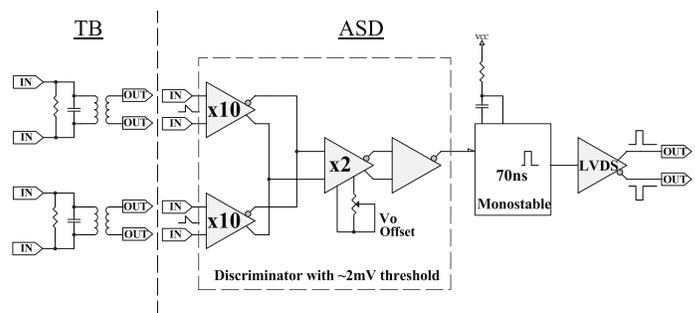
Fig. 3. A schematic for the signal processing that occurs on the Transition Board (TB) and Amplifier-Shaper-Discriminator board (ASD). The  $RC$  circuit ( $R = 150 \Omega$ ,  $C = 12$  pF) in parallel with a transformer (1:1) on the TB is designed to reduce noise and reflection problems at the input ( $Z = 50 \Omega$ ). On the ASD the amplifiers and comparator effectively sum the two PMT signals and discriminate on the leading edge with a 2 mV threshold.
