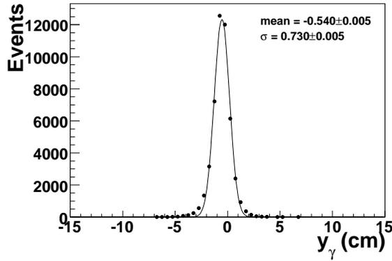
Fig. 17. The spectrum of reconstructed  $y_\gamma$  positions with the slit collimator inserted into the beamline. Note that the mean of the spectrum is consistent with the offset of the slit collimator centroid.
