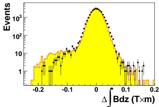
Fig. 21. The spectrum obtained from observed  $e^+e^-$  conversions for the integrated field calculated from the events' measured energies and positions minus the nominal integrated field. The nominal value is  $\int Bdz \sim 0.32$  Tm.
