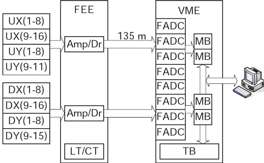
Fig. 5. Schematic of the luminosity spectrometer DAQ system. The calorimeter signals are sent to the nearby FEE system. The analog signals then travel to the ZEUS hall to be processed by the digital system in a VME crate.
