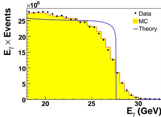
Fig. 22. The observed spectrum corrected for acceptance (multiplied by  $E_\gamma$ ) as a function of  $E_\gamma$  for the magnet current raised so as to observe the spectrum end point. The continuous curve specifies the spectrum shape predicted for a perfect detector. The histogram shows the Monte Carlo prediction for this detector.
