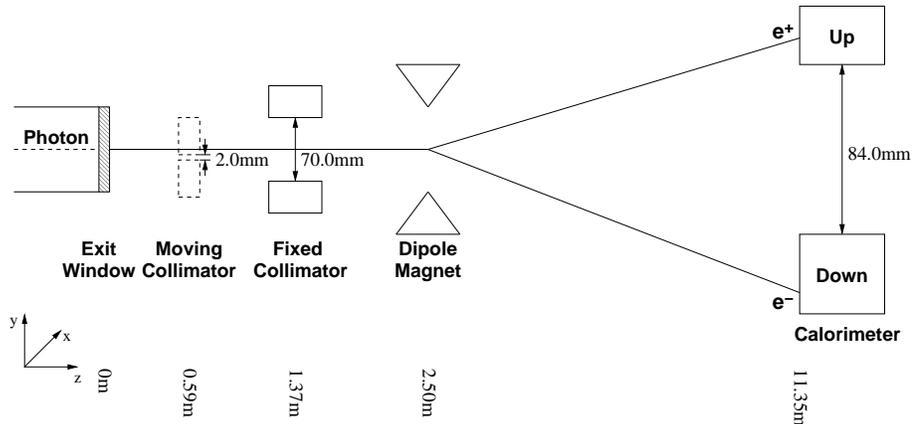
Fig. 1. Schematic showing major elements of the luminosity spectrometer. Note the very different scales for transverse and beam directions, and note that the exit window is 92.5 m downstream of the  $ep$  nominal interaction point. The origin for the transverse coordinates ( $x, y$ ) was chosen at the center of the exit window.
