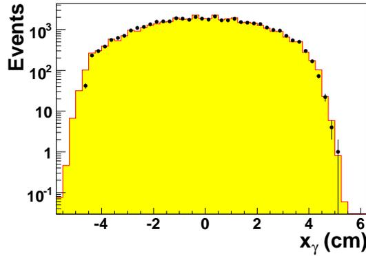
Fig. 19. The spectrum of reconstructed  $x_\gamma$  positions for accepted photons shown on a logarithmic scale. The Monte Carlo predictions are shown as the histogram. Note the high statistics of the data, which were collected in one 16 second period.
