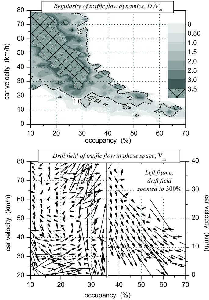
**Fig. 3.** Structure of ensemble vehicle dynamics in the phase space  $\{o, v\}$ . The upper window visualizes distribution of ratio between the random and regular components of the effective forces. The lower window depicts the regular drift field.
