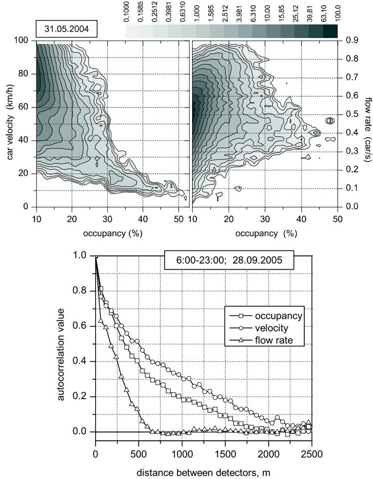
**Fig. 2.** Fundamental diagrams (upper frames) and autocorrelations in the occupancy, car velocity, and flow rate measured by differing detectors vs the distance between them (lower frame).
