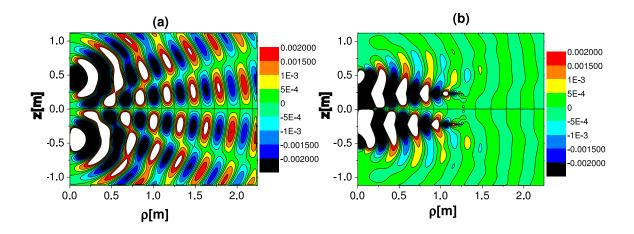
Fig. 3. (Color online) Distribution of the azimuthal magnetic field component  $H_{\varphi}(\rho,z)$  in the absence of the LHM disc  $(R_L=0,\ P_{in}=P_r=14.22\,mW)$  (a) and in its presence  $(R_L=1.27\,m,\ v/\omega=0.005,\ P_{in}=14.6\,mW,\ P_r=0.66\,mW)$  (b). The black/white color means large negative/positive values of the magnetic field.
