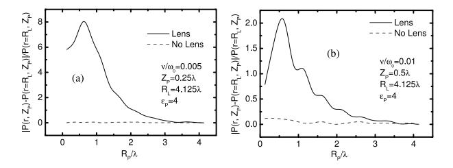
Fig. 5. Comparison between the relative changes in the total emitted power for a non-radiating configuration ("lens") and a pair of dipoles with no lens ("no lens") resulting from the presence of a ring (see Fig. 1) of dielectric permittivity  $\varepsilon_P = 4$  and  $D = \lambda/2$ , where  $\lambda$  is the excitation wavelength, as a function of the internal radius of the ring. The frequency is  $\omega = 1 \, \text{GHz}$ . The values of the other parameters are shown on the graphs.
