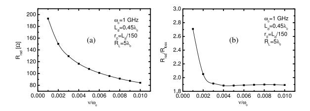
Fig. 7. Radiation and loss resistance for a system of wire dipoles coupled through a disc of LHM and fed with in-phase voltages. In the absence of any lens the radiation resistance of the dipole is 75  $\Omega$ . Radiation resistance as a function of the collision frequency in (a). The ratio between the radiation and the loss resistances as a function of the collision frequency in (b).
