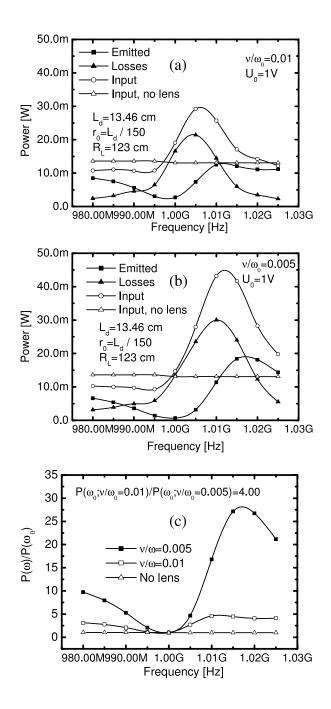
Fig. 4. Input power, radiated power and loss power as a function of the excitation frequency  $\omega$ . The frequency value at which the index of refraction of the LHM is equal to -1 is denoted by  $\omega_0$ . The value of the collision frequency is  $v/\omega_0=0.01$  (a) and  $v/\omega_0=0.005$  (b). The emitted power normalized to its value at  $\omega_0$  is shown on (c). For a comparison the behavior of the same pair of dipoles but in the absence of the lens is also shown.
