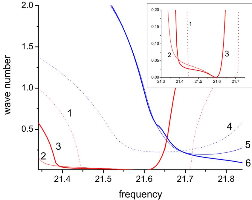
FIG. 4: Decay rates of  $29TM1$  (1, 2 and 3) and  $24TM2$  (4, 5, and 6) bands. The labelling of the curves is the same as in Fig.3. The insert shows, in a magnified form, the spectral region corresponding to  $29TM1$  mode. One can see a significant increase in the radiative decay rate of this mode in the vicinity of the new band boundaries, which, however, decreases to the initial WGM value at  $x = x_{29,1}$
