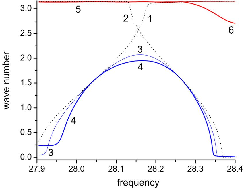
FIG. 6: Dispersion laws describing hybridized bands arising as a result of interaction between  $39TE1$  and  $34TE2$  supermodes. Curves 1 and 2 represents initial unperturbed dispersion laws, 3 and 5 are dispersion curves obtained without accounting for interaction with reservoir modes, and curves 4 and 6 depict dispersion laws of two branches with reservoir modes taken into account. The upper branch is almost completely pushed to the forbidden region.
