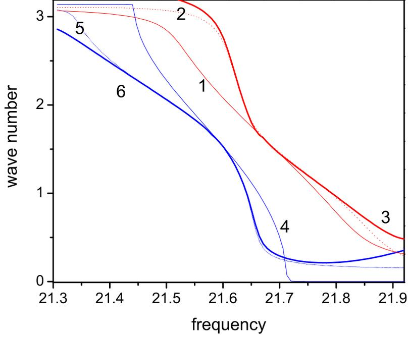
FIG. 3: Dispersion curves of  $29TM1$  and  $24TM2$  bands. Dash lines labelled 1 and 4 presents single-band dispersion curves, thin lines labelled 2 and 5 demonstrates dispersion cruves found without reservoir modes taken into account, and finally thick lines labelled 3 and 6 show dispersion curves with reservoir modes included
