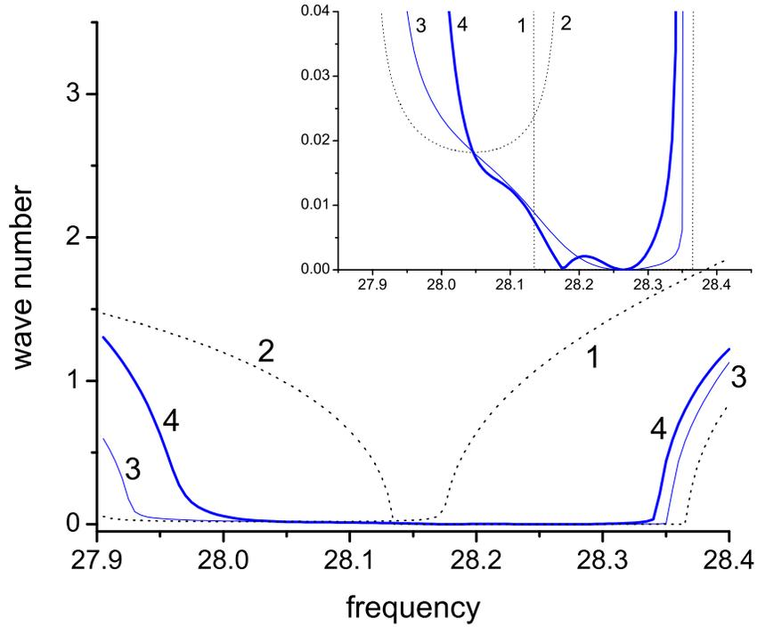
FIG. 7: Radiative decay rates for the allowed hybridized band. The labeling of the lines is the same as in Fig.6. The insert magnifies the region around the center of  $39TE1$  band.
