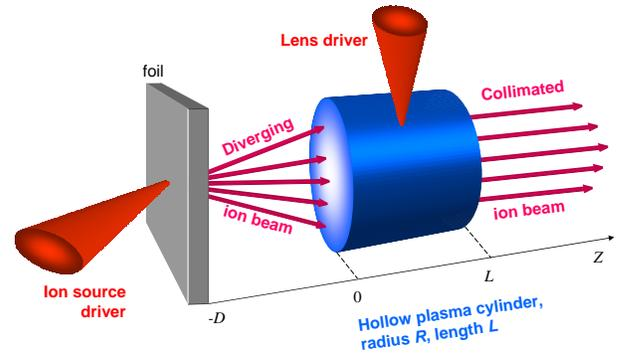
FIG. 1: (color online). Geometry of the ion optics element for focusing of laser-generated ion beams. One laser beam generates an ion beam from the rear side of the irradiated foil. Another laser beam hits a hollow cylinder, where a hot electron population is generated. The cylinder has the radius  $R$ , the length  $L$  and is located at the distance  $D$  from the foil. The radial electric field of the plasma inside the cylinder collimates the ion beam.
