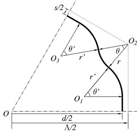
Fig. 2. Schematic diagram of a portion (1/6) of the improved PC unit. Thick line is air-silica interface, with air to its left.
