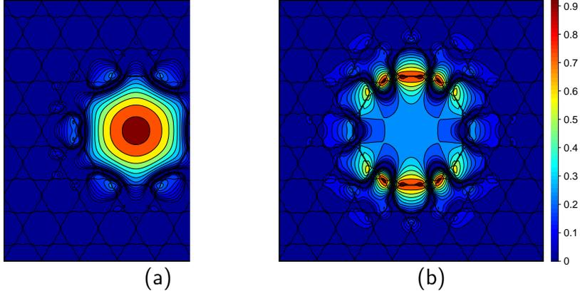
Fig. 4. Air-guided mode at  $\lambda = 1.55\mu\text{m}$  (a) and surface mode at  $\lambda = 1.30\mu\text{m}$  (b). Contour lines are in 1-dB separation.
