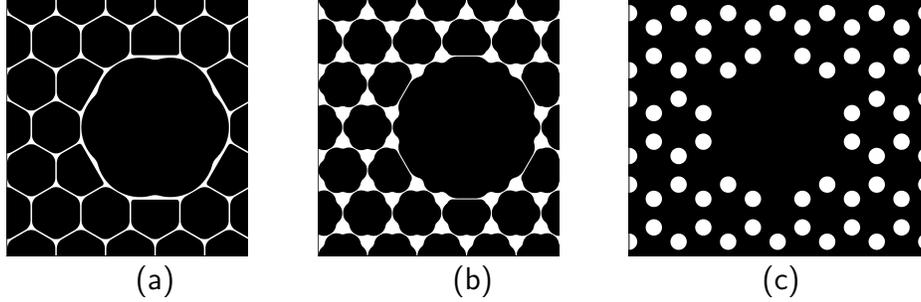
Fig. 1. (a) Air-guiding PCF reported in Ref. 2. (b) Proposed air-guiding PCF. (c) Ideal rods-in-air PCF. Black is for air.
