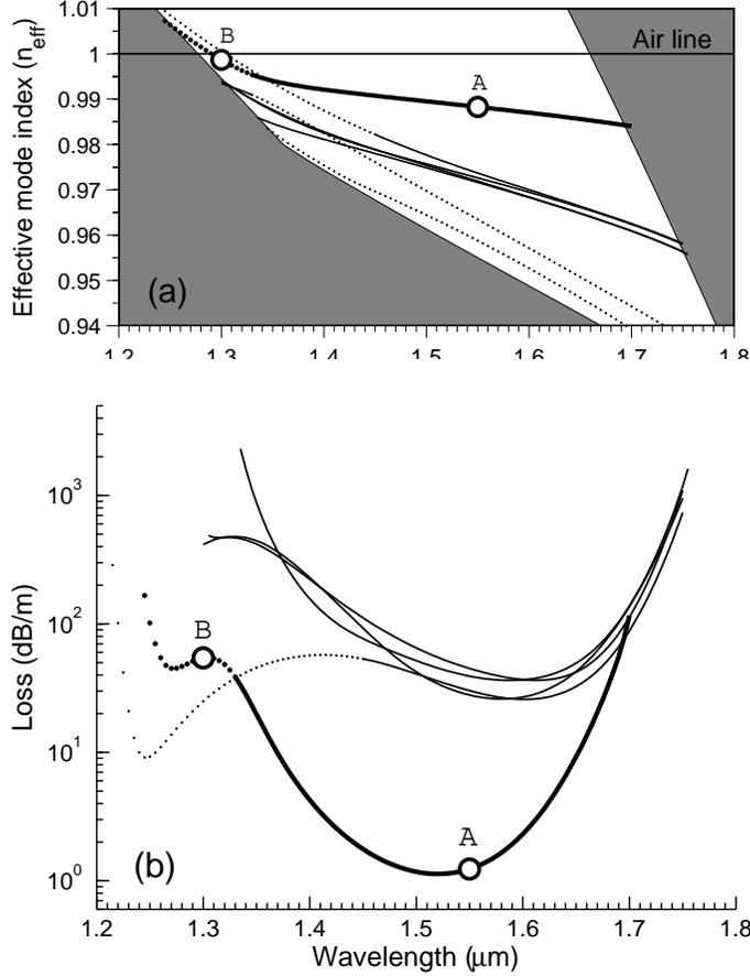
Fig. 3. Dispersion (a) and loss (b) curves of the defect modes. Photonic bandgap region of the cladding PC is represented by the white patch in (a).
