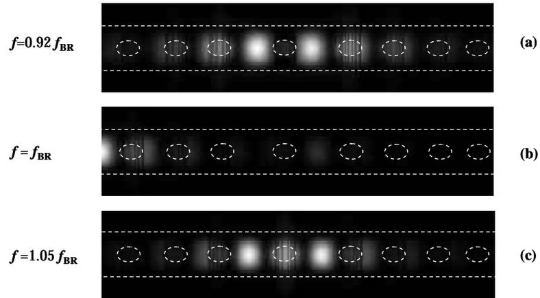
Fig.4. Simulated field intensity patterns in the  $xy$ -plane corresponding to the resonating modes (at frequencies  $f=0.92 f_{\text{BR}}$  and  $1.05 f_{\text{BR}}$ ) and at the Bragg frequency  $f_{\text{BR}}$  for the aperiodic lattice of Fig.3 (iv-a).
