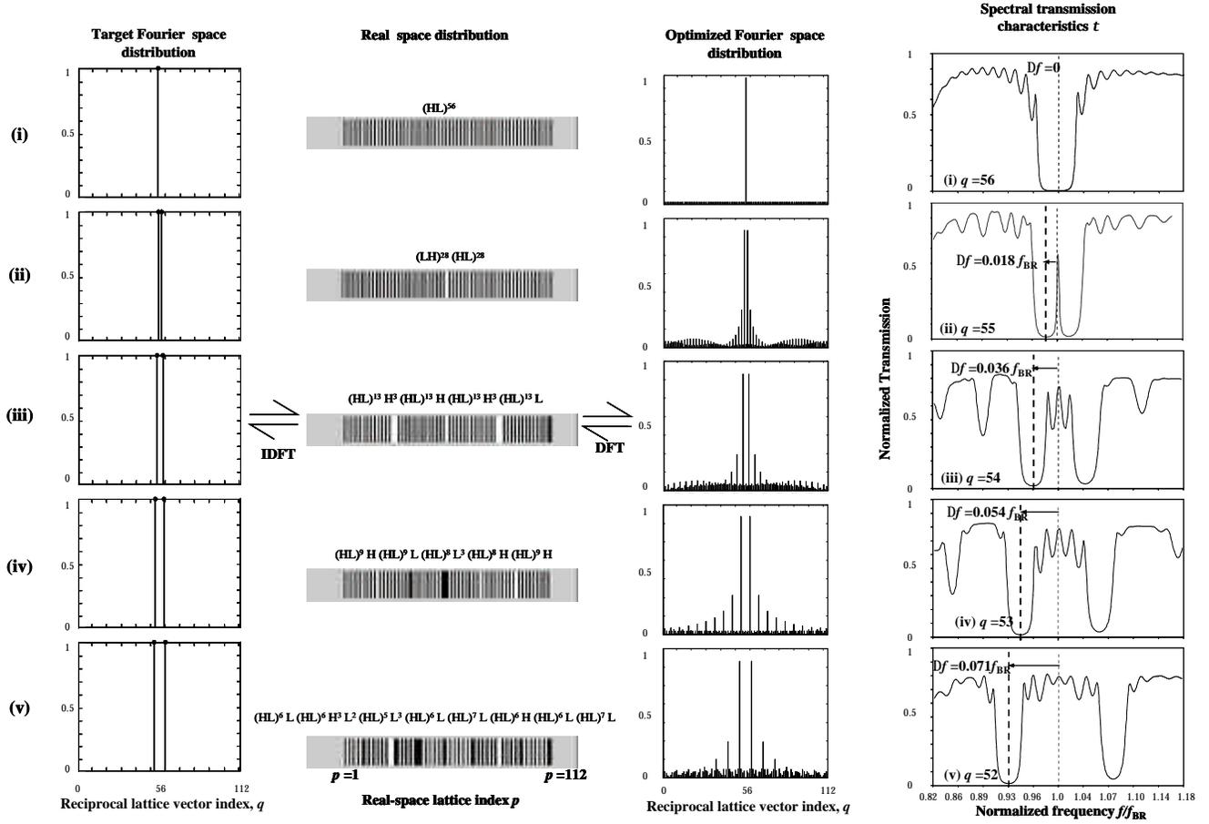
Figure 2. Optical transmission spectra (transmission  $t$  versus normalized frequency  $f/f_{BR}$ ), calculated using FIMMPROP-3D. Figures (i-v) show use of AL's to shift the PBG into the Brillouin Zone in steps of  $\sim 0.02 f_{BR}$  from the edge of the Bragg frequency  $f_{BR}$ .
