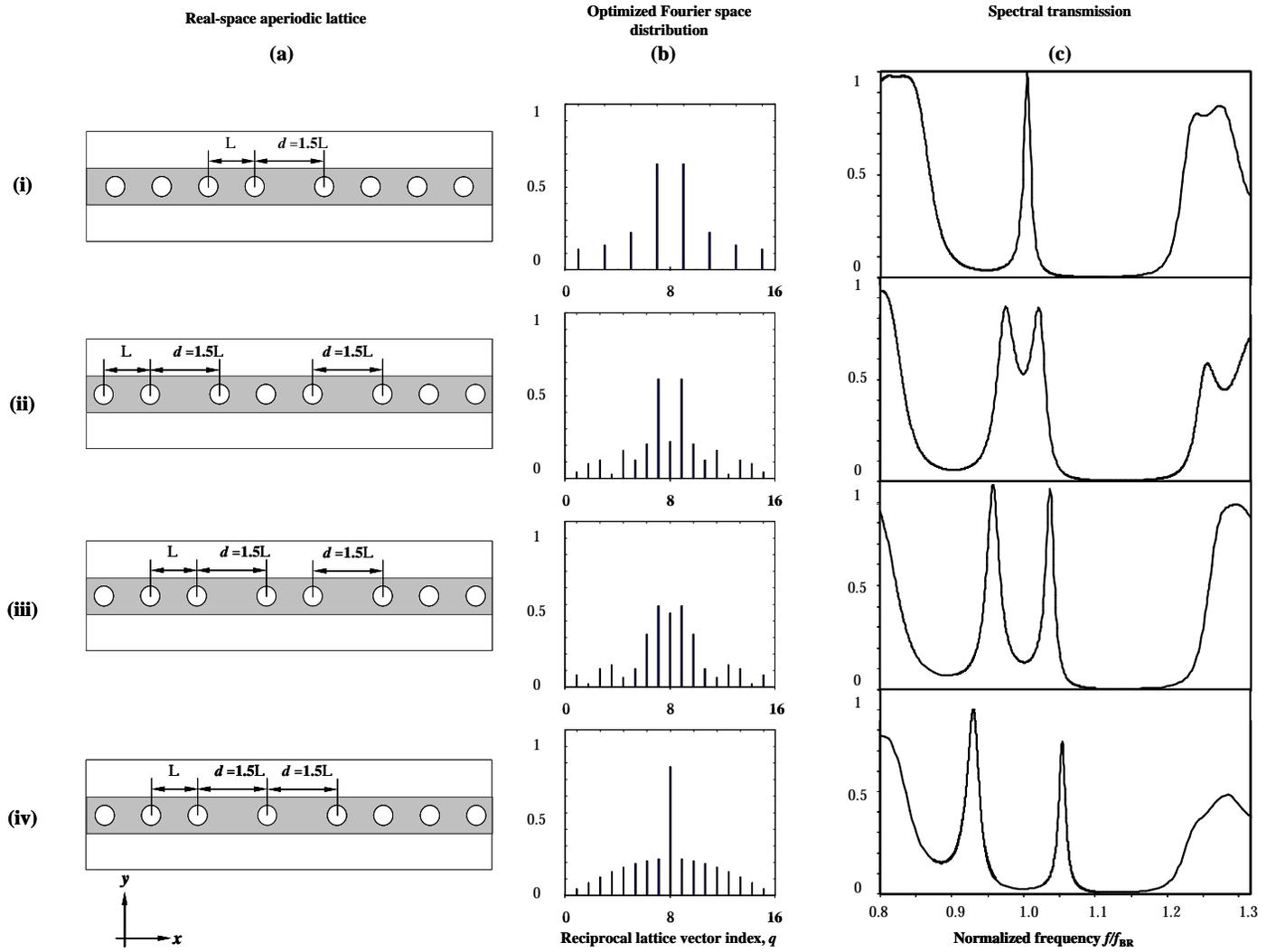
Fig.3. The Fourier component distributions and spectral transmission characteristics of four different aperiodic lattices doped with defects. We have used  $N=16$  unit-cells, with the normalised DFT Nyquist frequency ( $G_{BR}$ ) corresponding to  $q=N/2 = 8$ . Evident is the systematic progression from a single high-Q transmission peak to double high-Q transmission peaks.
