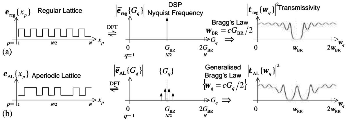
FIG. 1: Qualitative understanding of how we can combine simple rules of DSP with Bragg's Law, in order to predict the position of the dips in the electromagnetic transmission spectrum of any real AL.
