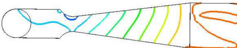
**Figure 8.** Isolines of static pressure at the middle-height cross-section of the channel at medium flow rate, computation, CFX-5
