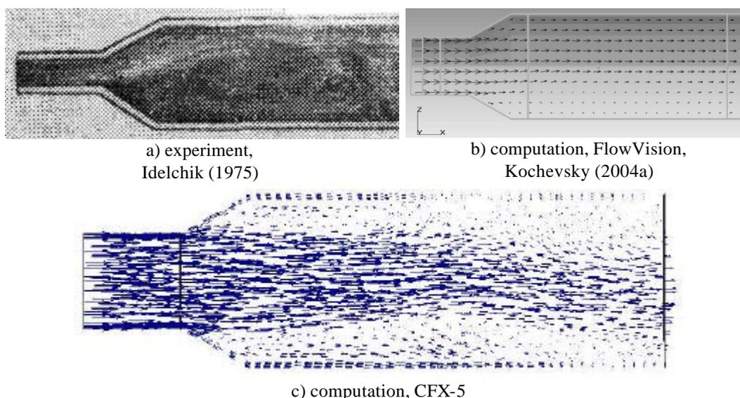
**Figure 1.** Instant flow pattern in a conical diffuser with area ratio 3.3 and internal angle  $60^\circ$
