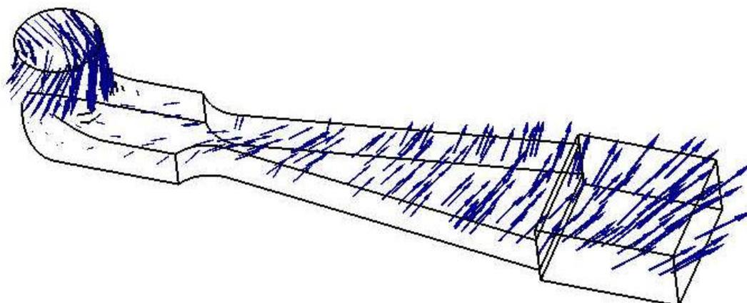
**Figure 10.** Velocity vectors of flow in relative motion (at the channel inlet) and in absolute motion (inside the channel and at the channel outlet) at medium flow rate
