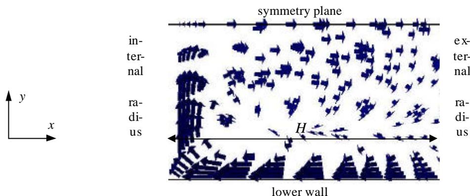
**Figure 4.** Velocity vectors at the cross-section corresponding to 90-degree angle of turn
