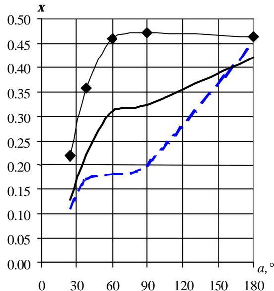
**Figure 2.** Dependence of loss factor on internal angle of a conical diffuser with area ratio 3.3: markers connected with the thin line – experiment, Idelchik (1975), dotted line – computation, FlowVision (Kochevsky, 2004a), solid line – computation, CFX-5
