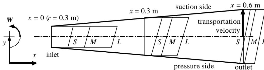
**Figure 7.** Velocity distribution in the channel according to the potential flow analysis: S – low flow rate (average velocity at the outlet cross-section of the channel is 2.8 m/s), M – medium flow rate (5.3 m/s), L – high flow rate (11.0 m/s)
