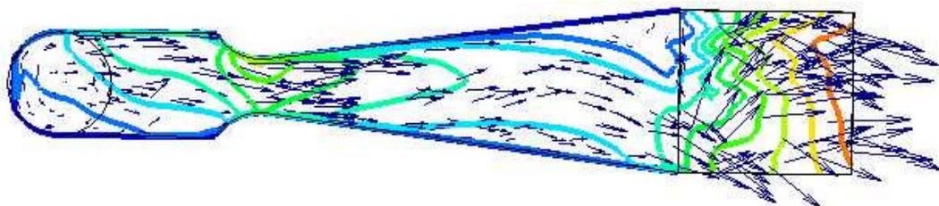
**Figure 9.** Velocity isolines and vectors in relative motion at medium flow rate, computation, CFX-5. At the upper right corner, near the channel outlet, a stagnation zone is seen
