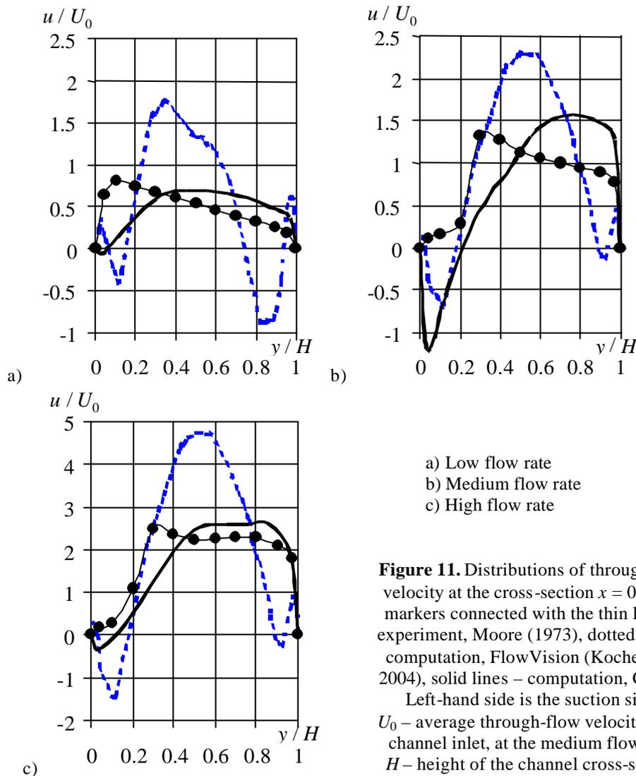
**Figure 11.** Distributions of through-flow velocity at the cross-section  $x = 0.46$  m: markers connected with the thin lines – experiment, Moore (1973), dotted lines – computation, FlowVision (Kochevsky, 2004), solid lines – computation, CFX-5. Left-hand side is the suction side.  $U_0$  – average through-flow velocity at the channel inlet, at the medium flow rate,  $H$  – height of the channel cross-section
