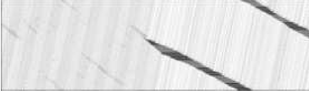
Fig. 25. A time-space diagram of the VDR-TCA model for v_{\max} = 5 cells/time step, p_0 = 0.5 , p = 0.01 , and a global density of k = \frac{1}{6} vehicles/cell. The shown lattice contains 300 cells, with a visible period of 1000 time steps. We can see the breakdown of an initially homogeneous traffic pattern. As the phase separation takes place, a persistent compact jam is formed, surrounded by free-flow traffic. The significant decrease of the density in the regions outside the jam results from the jam's reduced outflow.
