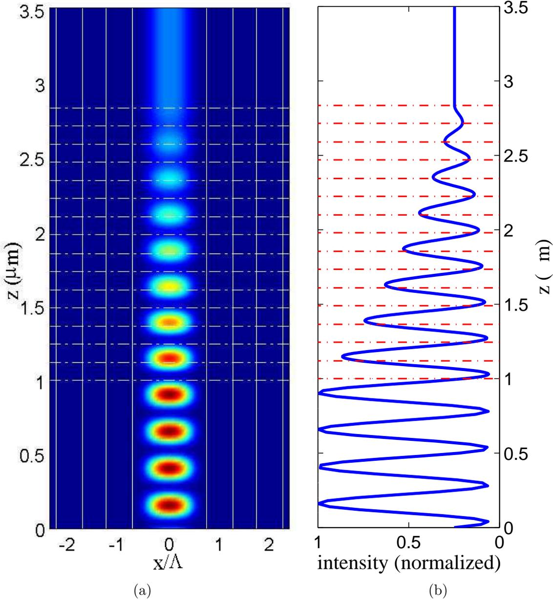
**Figure 7.** Distribution of electric field intensity (a) on the  $xz$  plane at the center of the fibre core and (b) at the center of the fibre core.
