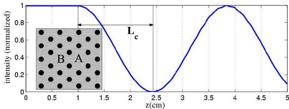
**Figure 4.** Intensity of electric field in the center of the core A. The inset shows the cross section of the PCF coupler with the two cores A and B.
