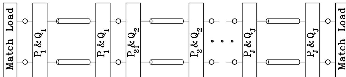
**Figure 3.** Equivalent transmission-line network of the multi-layered structure shown in Fig. 1.
