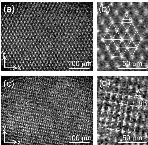
FIG. 4: Images of a cold ensemble of  $\sim 13,000$  ions. (a) Visible hexagonal structures indicating a three-dimensional bcc structure. (b) Magnification of a section of (a). The side length  $d$  is found to be  $17.2 \mu\text{m}$ . (c) Visible rectangular structure likely indicating a slightly distorted fcc structure. (d) Magnification of a section of (c). Here,  $h = 15.2 \pm 0.5 \mu\text{m}$  and  $w = 9.71 \pm 0.2 \mu\text{m}$ , respectively.
