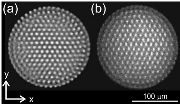
FIG. 3: Images of Coulomb crystals. (a) Time averaged image based on data from MD simulations of Coulomb clusters with 2685 ions at  $\Gamma \sim 400$  (temperature:  $\sim 5$  mK). The averaging time is 10 ms. (b) Image from experiments with clusters containing  $\sim 2700$  ions.
