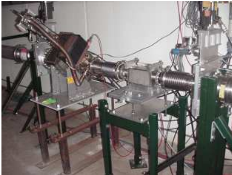
Fig. 3. Photograph of the prototype segmented Foil SEM installed in the 8 GeV beamline.
