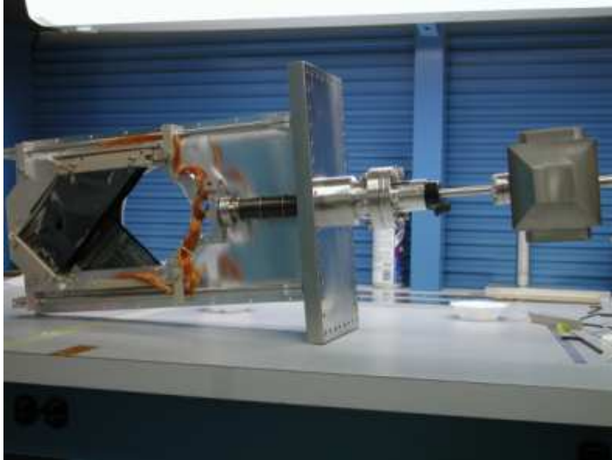
Fig. 2. Photograph of the prototype segmented Foil SEM. At right is the signal connection feedthrough box. At center is the lid of the vacuum chamber for the SEM, and at left is the paddle with the foils. The foil paddle moves in and out of the beam on rails, and the vacuum during the motion is maintained by a bellows feedthrough mounted to the vacuum chamber lid. The assembly shown is approximately 75 cm long by 30 cm tall.
