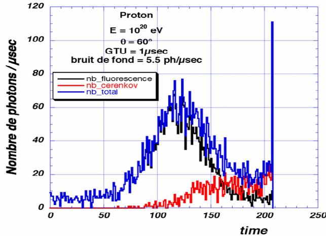
**Figure 1.** Left: time distribution of the photons per pixel arriving at the EUSO focal surface for a proton shower of  $E=10^{20}$  eV with an incidence angle of  $60^\circ$ . The fluorescence and Cerenkov contributions are distinguished. The black histogram corresponds to the photons flux if the atmosphere was totally transparent. A GTU is a Gate Time Unit.
