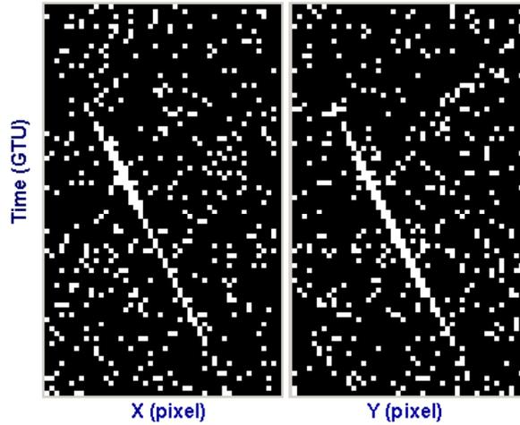
**Figure 5.** Schematic view of a track along the two projection view (as registered by the read-out electronics). Shower simulated at energy  $E = 10^{20}$  eV and arrival direction zenith angle  $\sim 60^\circ$ .
