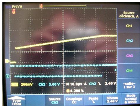
**Figure 4.** Voltages (white track) created with a DAC controlled by the computer. Here, a ramp followed by a plateau was made.
