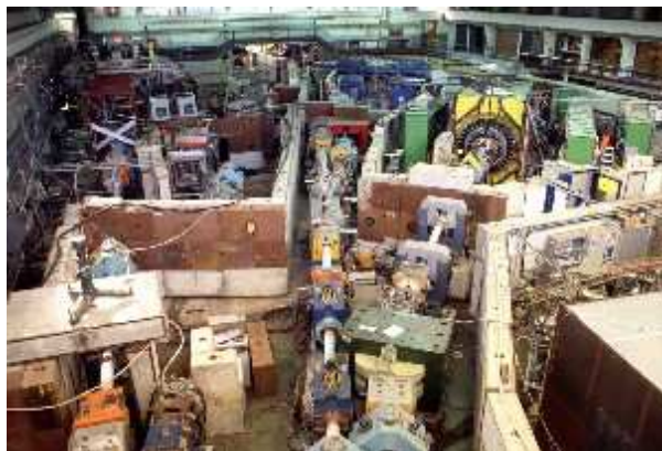
Figure 1: Overview of the LEAR experimental area. The Low Energy Antiproton Ring (LEAR) at CERN, is the only one of its kind in the world. It enables scientists to study the details of antiproton interactions with the nucleus of atoms. In the picture we can see the 80 meter in circumference ring that permits the storage and slowing of antiprotons down to energies as low as 5 MeV. It's the first machine ever built to decelerate, rather than accelerate, particles. (Photograph: CERN Bulletin 47/98, 16 November 1998.)
