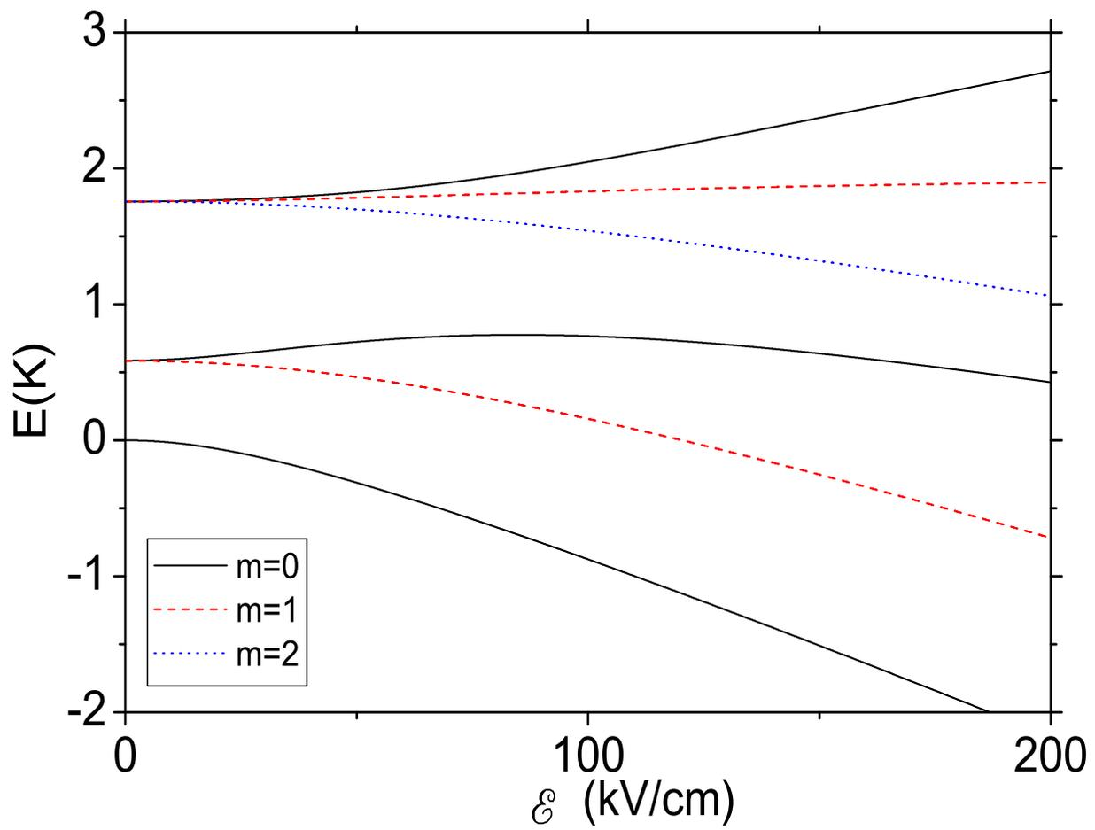
FIG. 1: Stark effect for linear OCS molecules in their  $^1\Sigma$  ground state.
