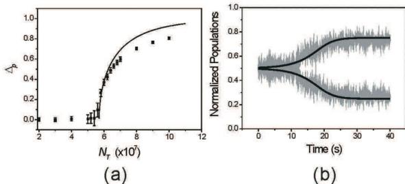
FIG. 4: (a)  $\Delta_p$  vs  $N_T$ , obtained by Monte-Carlo simulations with  $10^3$  atoms. The solid curve is a plot of Eq. (3). (b) Simulation curves for the temporal evolution of SSB, in good agreement with the experimental data (Fig. 2(b)). Here  $W_0 = 1.0 \text{ s}^{-1}$  and  $N_T = 1.1N_c$ .
