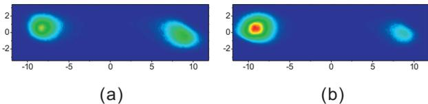
FIG. 1: Snapshot images of atoms in two dynamic attractors (a) before SSB of atomic population and (b) after SSB, taken by a charge-coupled-device (CCD). The total number of atoms is (a)  $6.1 \times 10^7$  and (b)  $6.9 \times 10^7$ , respectively. The relative population difference in (b) is 0.63. Here  $f = 96$  Hz,  $h = 0.9$ , and the abscissas are in unit of mm.
