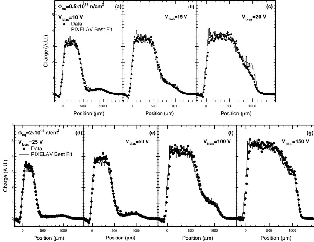
Fig. 3. Measured (full dots) and simulated (histogram) charge collection profiles for a sensor irradiated to a fluence of  $\Phi = 0.5 \times 10^{14} \text{ n}_{\text{eq}}/\text{cm}^2$  (a-c) and of  $\Phi = 2 \times 10^{14} \text{ n}_{\text{eq}}/\text{cm}^2$  (d-g), and operated at several bias voltages.
