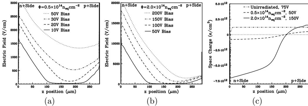
Fig. 4. The  $z$ -component of the simulated electric field resulting from the model best fit is shown as a function of  $z$  for a sensor irradiated to a fluence of  $\Phi = 0.5 \times 10^{14} \text{ n}_{\text{eq}}/\text{cm}^2$  (a) and  $\Phi = 2 \times 10^{14} \text{ n}_{\text{eq}}/\text{cm}^2$  (b). (c) Space charge density as a function of the  $z$  coordinate for different fluences and bias voltages.
