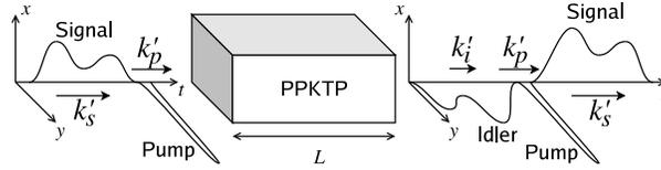
Fig. 1. Schematic of spectral phase conjugation (SPC) via type-II extended phase matching (EPM). The signal and idler pulses, in orthogonal polarizations, have carrier frequencies of  $\omega_s$  and  $\omega_i$ , while the pump pulse has a carrier frequency of  $\omega_p = \omega_s + \omega_i$ . The EPM condition requires that the signal and the idler counterpropagate with respect to the pump, which should be much shorter than the input signal.
