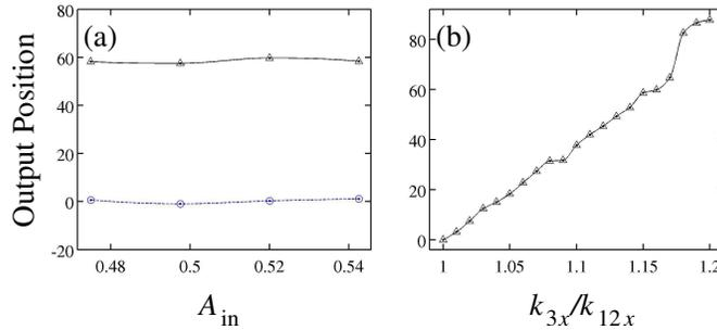
Fig. 4. Output soliton position vs. (a) the amplitude of the input Gaussian beam and (b) the angle between the modulating beam and the lattice-forming beams, defined by the ratio  $k_{3x}/k_{12x}$ . Dashed line and circles correspond to Fig. 2(a), solid lines and triangles – to Fig. 2(b). Parameters are the same as in Fig. 2.
