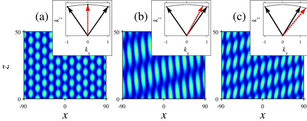
Fig. 1. Examples of one-dimensional photonic lattices modulated by the third beam with the transverse wave number  $k_{3x}$ : (a)  $k_{3x} = 0$ , (b)  $k_{3x} = 0.8k_{12x}$ , and (c)  $k_{3x} = 1.3k_{12x}$ . Insets show the wave vectors of two input beams which form the lattice, and the wave vector of the third beam (red, dashed). Parameters are  $A_{12} = 0.25$ ,  $A_3 = 0.66A_{12}$  and the propagation length is  $L = 50$  mm.
