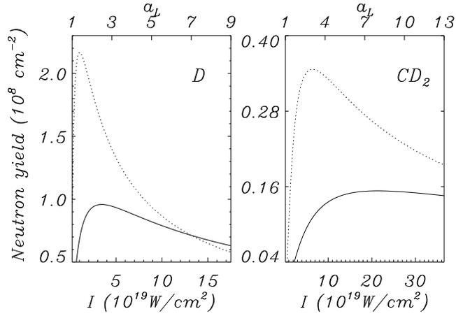
**Fig. 3** Analytical scaling of the number of neutrons (per unit surface) produced during the ultrashort burst as a function of laser intensity for a  $\lambda = 0.8 \mu\text{m}$  pulse, for a “D” target with  $n_e = 40n_c$  and a “CD<sub>2</sub>” target with  $n_e = 250n_c$ . Solid and dotted curves correspond to the choice of “flat-top” and monochromatic distribution functions, respectively.
