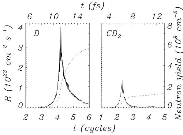
**Fig. 2** Numerical evaluation of the rate (solid line) and the total number (dotted line) of neutrons produced per unit surface for the “D” simulation of Fig.1 (left panel) and for the “CD<sub>2</sub>” simulation for which  $n_e = 250n_c$ ,  $a_L = 8$ .
