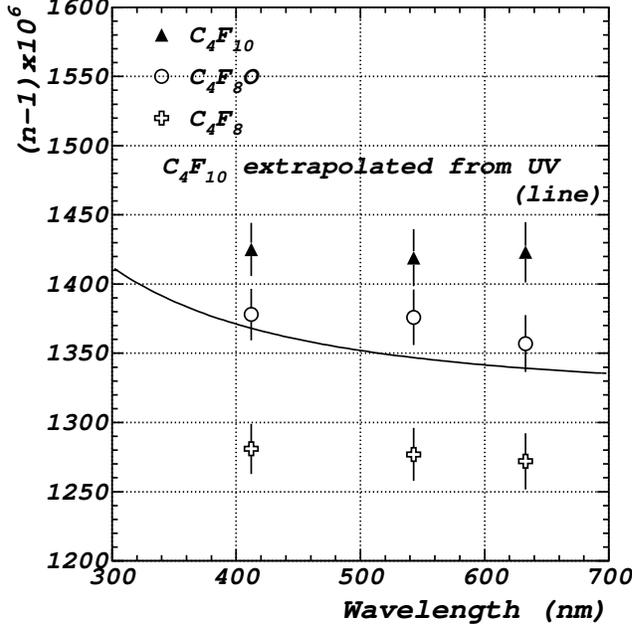
Fig. 18. Our measurement of the index of refraction of three gases corrected to 1 atmosphere pressure and 22°C nominal temperature. The curve is an extrapolation of  $C_4F_{10}$  measurements at shorter wavelengths that is used in the simulation.
