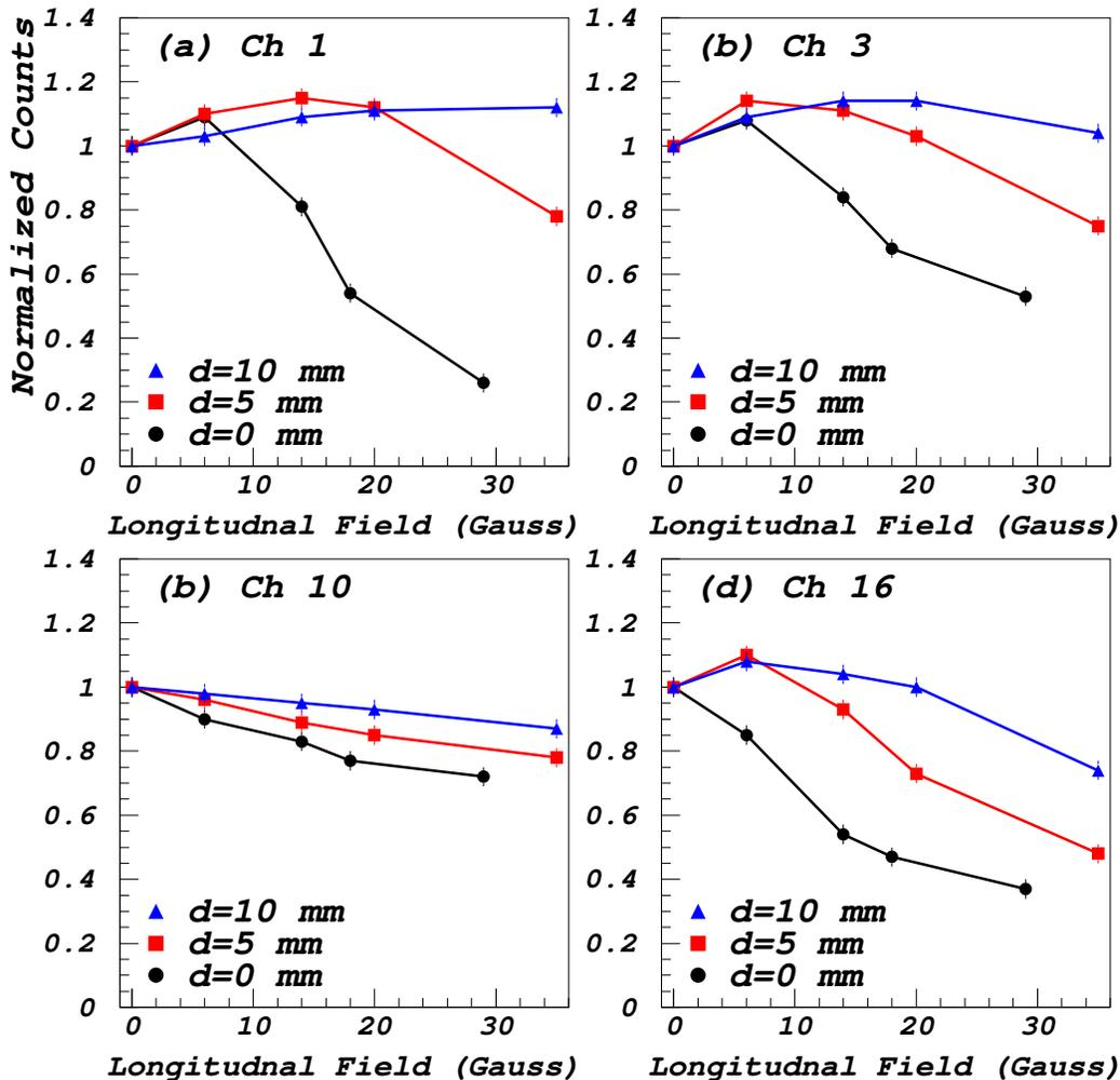
Fig. 13. Count rate as a function of the applied longitudinal magnetic field for shield extension values,  $d=0$  mm, 5 mm, and 10 mm, for (a) Channel 1, (b) Channel 3, (c) Channel 10, and (d) Channel 16.
