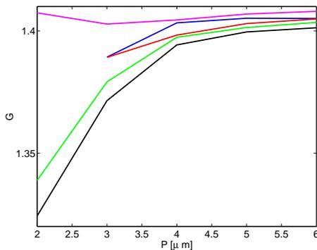
FIG. 4: The amplification of the pulses after propagating 10 cm in the fiber amplifier for the different fiber geometries:  $d/P = 0.2$  (magenta curve),  $d/P = 0.3$  (blue curve),  $d/P = 0.4$  (red curve),  $d/P = 0.5$  (green curve), and  $d/P = 0.6$  (black curve) as a function of the period  $P$ .
