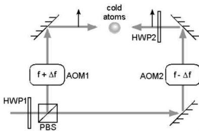
FIG. 1: Diagram of apparatus. The half-wave plate HWP1 and polarizing beam splitter PBS are used to create two equal intensity beams which are shifted in frequency by  $f \pm \Delta f$  by the AOMs. HWP2 is used to make the polarizations of the two beams parallel.
