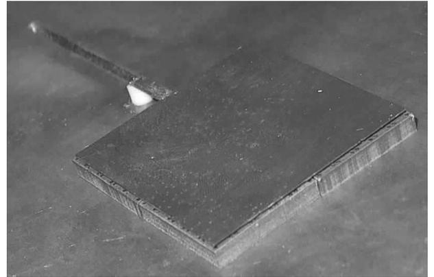
Fig. 12. Photo of the measured antenna filled with an artificial magnetic layer.
