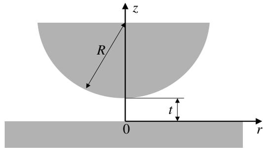
FIG. 1: Schematic presentation of the nanoscale junction consisting of a planar surface and a spherical asperity with curvature radius  $R$ , separated by the distance  $t$ . The fluid is nonuniformly distributed in the junction. The model resembles AFM tip dwelling above a sample surface.
