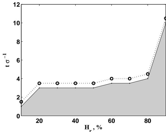
FIG. 2: Water condensation between planar surface and spherical asperity of the radius  $R = 36\sigma$  (10 nm). Shaded area corresponds to the formation of liquid meniscus. No liquid bridge is formed for given  $H_r$  when  $t$  reaches ordinate of the open circle. The parameters of fluid interaction with confining walls are  $\epsilon_s \epsilon^{-1} = 1$  and  $\alpha\sigma = 2$ .
