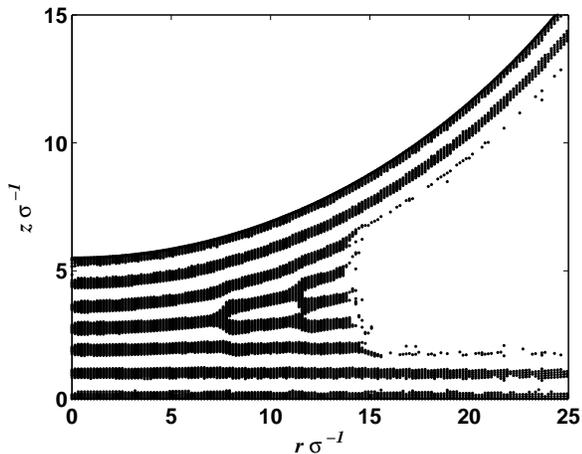
FIG. 4: Water meniscus formed between planar surface and spherical asperity of the radius  $R = 36\sigma$  (10 nm), separated by  $t = 5.5\sigma$ . Relative humidity is 90%, and parameters of fluid interaction with solid walls are  $\epsilon_s \epsilon^{-1} = 1$  and  $\alpha\sigma = 2$ .
