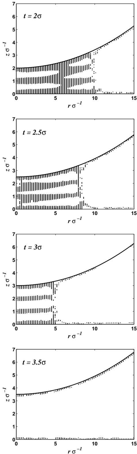
FIG. 6: Variation of the meniscus size with separation  $t$  between confining surfaces. Filled space on the plots corresponds to the regions where fluid density exceeds the threshold value of  $\sigma^3 \rho_{th} = 0.16$ . Relative humidity is 50%, and parameters of fluid interaction with solid walls are  $\epsilon_s \epsilon^{-1} = 1$  and  $\alpha\sigma = 2$ . Curvature radius of the asperity is  $R = 36\sigma$ .
