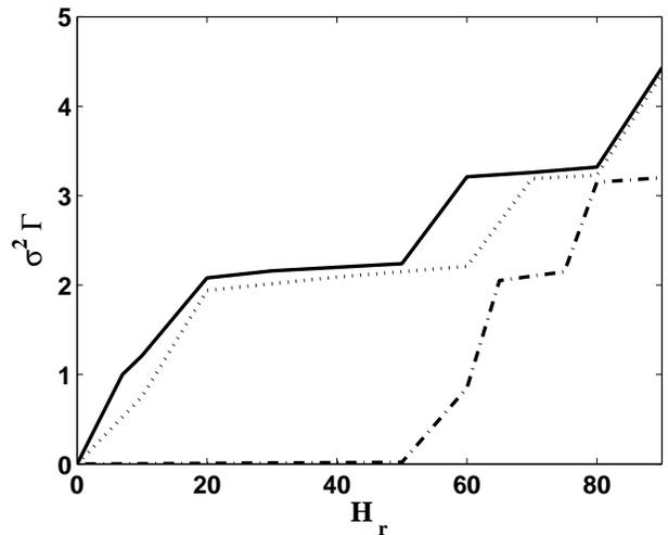
FIG. 7: Calculated adsorption isotherms for the model fluid on surfaces with different values of  $\epsilon_s \epsilon^{-1}$ : 1 (dash-dot line), 1.5 (dotted line), 2 (solid line), and with  $\alpha\sigma = 2$ .  $\Gamma$  is number of molecules adsorbed per unit surface area. As  $H_r$  approaches 100%, the onset of (integrable) singularity is observed (not shown).
