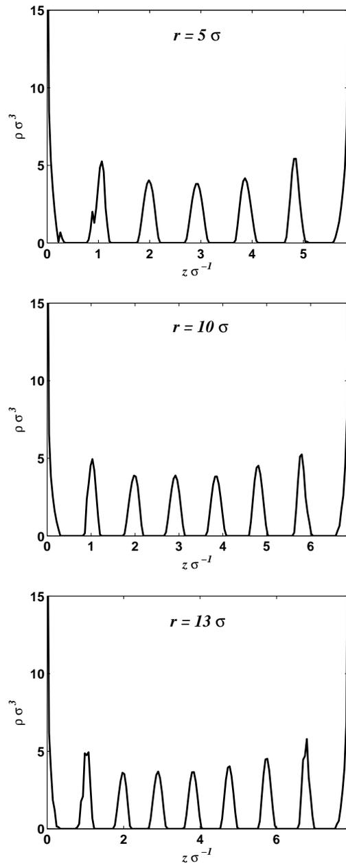
FIG. 3: Fluid density profiles between planar surface and spherical asperity of the radius  $R = 36\sigma$  (10 nm), separated by  $t = 5.5\sigma$ , for three different values of the radial coordinate  $r$ . Relative humidity is 90%, and parameters of fluid interaction with solid walls are  $\epsilon_s \epsilon^{-1} = 1$  and  $\alpha\sigma = 2$ .
