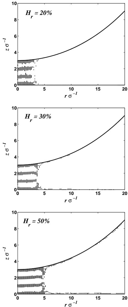
FIG. 5: Variation of the meniscus size with relative humidity  $H_r$ . Filled space on the plots corresponds to the regions where fluid density exceeds the threshold value of  $\sigma^3 \rho_{th} = 0.16$ . Other relevant parameters are:  $t = 3\sigma$ ,  $\epsilon_s \epsilon^{-1} = 1$  and  $\alpha\sigma = 2$ . Curvature radius of the asperity is  $R = 36\sigma$ .
