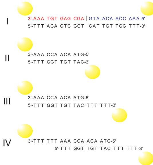
Fig. 1. DNA sequences used to form DNA-linked gold nanoparticles. Sample I is connected through a linker DNA. The line between bases A and G in the probe DNA sequences indicates that there is no chemical bond between these two bases. Sample II-IV are directly connected through surface-attached DNA with spacings of 12, 18, and 24 DNA bases between particles.
