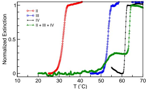
Fig. 3. Melting curves of 12/12 (sample II), 12/18 (sample III), 18/18 (sample IV), and a combination of 12/12, 12/18, and 18/18 (Sample II + III + IV). The mixed system shows multi-step melting at temperatures corresponding to the  $T_m$ 's, within the experimental uncertainty, for Sample II and Sample III.
