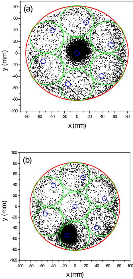
Figure 6. Reconstructed position of the scintillation points due to 122 keV  $\gamma$ -rays from a  $^{57}\text{Co}$  source, placed at the bottom of the chamber below the central collimator hole (a), and below a non-central position (b). The large circle corresponds to the active volume of liquid xenon scintillator, medium circles outline the photomultipliers and the small circles indicate the holes in the collimator, all to scale.
