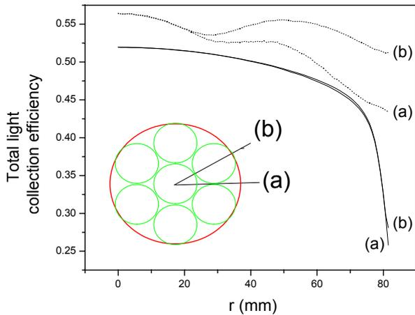
Figure 5. Total light collection efficiency, obtained by Monte Carlo simulation, as a function of the distance to the chamber axis along radial paths (a) and (b), as indicated in the insert. Solid lines are for  $z=0$  and dashed lines are for  $z=39$  mm (see Fig. 1). For  $z=0$  the light collection efficiencies for the two paths practically coincide.
