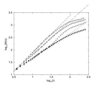
**Fig. 10.** Log log representation of the average mass M(r) measured within circle of radius r applied to the three cavities displayed in figure 9. Cirlcle, squares and diamonds are respectively for cavities 1, 2 and 3. Triangles up and left are for the right and left sides of the cavity (3) displayed in Fig. 9. The long dashed, the dot dashed and the dahed lines have respectively a slope of 1.5, 1.35 and 1.
