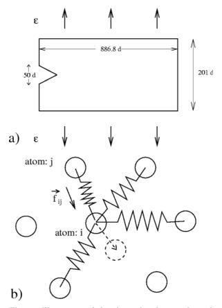
**Fig. 1.** Illustration of the elastic bond network used in the simulations. *a*) shows the specimen submitted to an external uniaxial tension . *b*) is a detailed view of the material consisting of atoms initially placed on a triangular lattice and connected by identical elastic springs. Note that a fixed density of springs is removed before application of the load.
