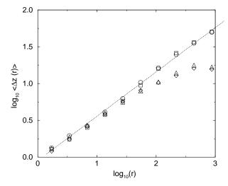
**Fig. 8.**  $log_{10}(\langle \Delta z(r) \rangle)$  as function of  $log_{10}(r)$ . Circles and squares show the result of the analyse of the top and bottom profiles after failure at  $T^*=80$  while diamonds and triangles are obtained when top and bottom failure profiles obtained at  $T^*=8$  are considered. These results where shifted verticaly for convinience. The dotted line has a slope of 0.6.
