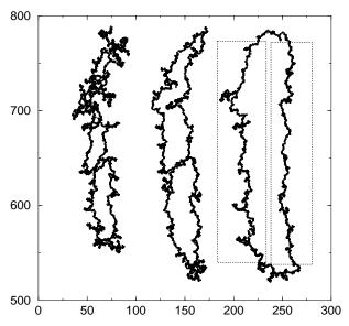
**Fig. 9.** From the left to the right, pictures of the same cavity at stages (1), (2) and (3) of the test performed on the porous material at temperature 80. The distance from the crack tip is respectively: 393, 359 and 355 atoms spacing. The boxes indicate the left and right sides of the cavity at stage (3).
