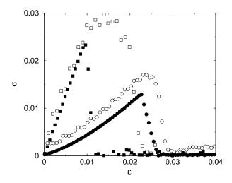
**Fig. 2.** Stress-strain evolution of the system. Circles and squares correspond respectively to c=0.3 and c=0 (non-porous material). Filled and empty symbols correspond respectively to  $T^*=8$  and 80.
