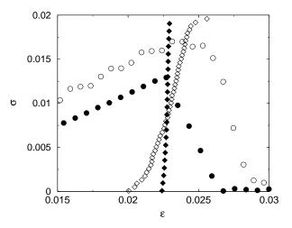
**Fig. 5.** Filled and unfilled symbols correspond respectively to  $T^* = 8$  and 80. Circles show the stress-strain variation for a porosity c = 0.3. Diamonds show the number of broken bonds vertically normalised to fit the plot.
