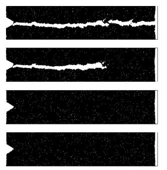
**Fig. 3.** Breakdown of the atoms network under strain test performed at the temperature  $T^*=8$ . From bottom to top the strain is respectively  $\epsilon=0.0223,\ 0.0224,\ 0.0225$  and 0.0282.
