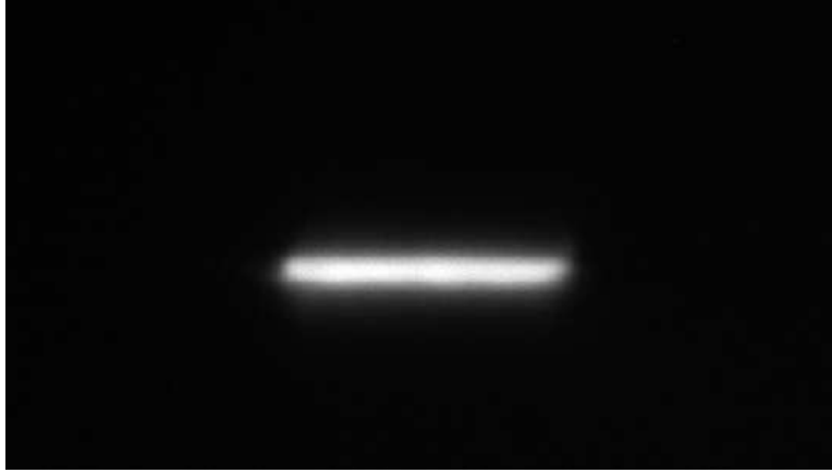
Figure 4-35: Atom fluorescence imaged by microscope in side imaging configuration. Similar but smaller images were used to measure atomic density during the experiment.
