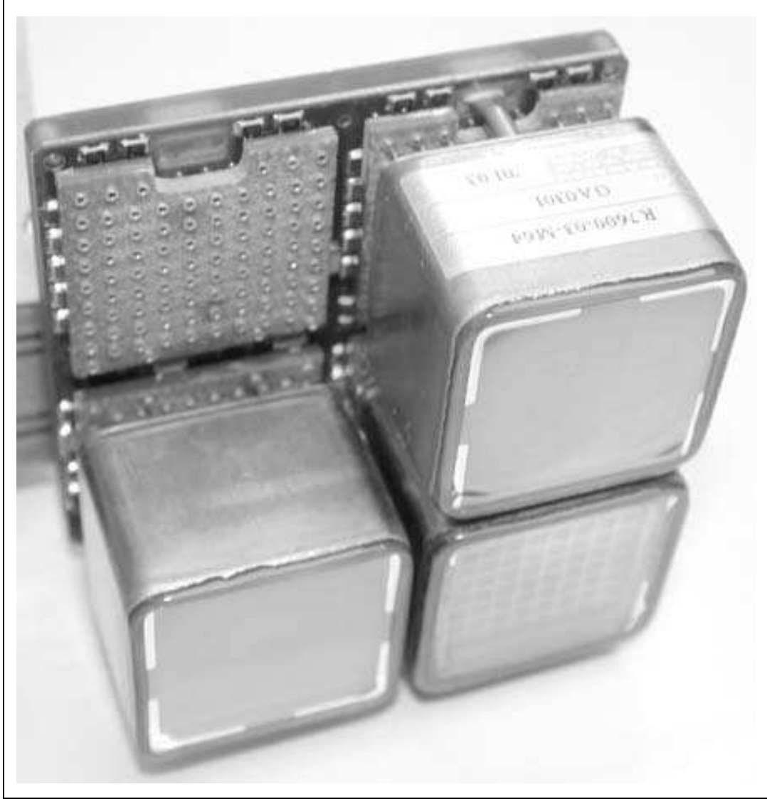
Fig. 4. Front-view of the prototype EC, with three of the MAPMT installed but without Light Collector Systems and no potting.
