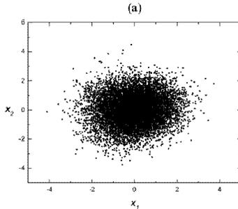
FIG. 5: Phase-space distribution for the period-one state from the multi-particle tracking for the linear wake function. The parameters are given as  $T_e = 10$ ,  $\nu = 0.25$ ,  $b = 0.25$  and 20,000 turns. The equilibrium state shows the same distribution per turn.
