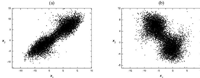
FIG. 6: Phase-space distribution for the period-two state from the multi-particle tracking for the composite wake function. The parameters are given as  $\nu = 0.20$ ,  $T_e = 22$ ,  $a = 8$  and  $b = 0.18$ . (a) and (b) shows the phase space distributions at 19,999 and 20,000 turns, respectively. The equilibrium state shows the same distribution per two turns.
