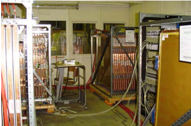
Figure 8 - A picture of the test room with 120 chambers connected to Gas, HV and readout.
