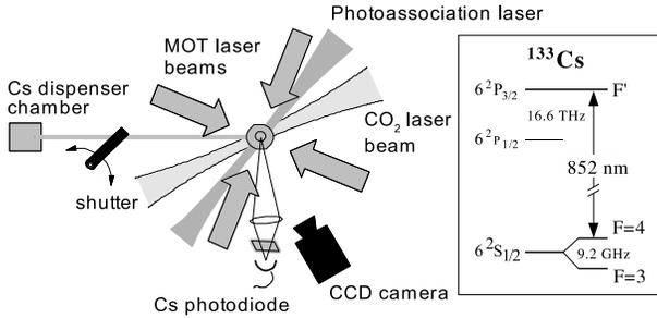
**Fig. 2** Experimental setup consisting of a cesium magneto-optical trap overlapped with a  $\text{CO}_2$  optical dipole trap and a photoassociation laser.
