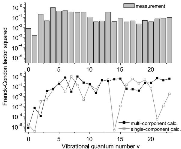
**Fig. 6** Experimental data (upper panel) and theoretical results (lower panel) for the square of the Franck-Condon factor as a function of the vibrational level for photoassociation resonances into  $J = 2$  states in the  $0_g^-$  outer well. Each curve is normalized to the maximum Franck-Condon factor.
