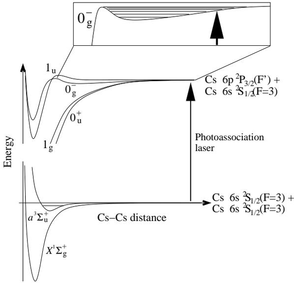
**Fig. 1** Schematic overview of the relevant molecular potential curves for  $\text{Cs}_2$  photoassociation into the  $0_g^-$  outer well.
