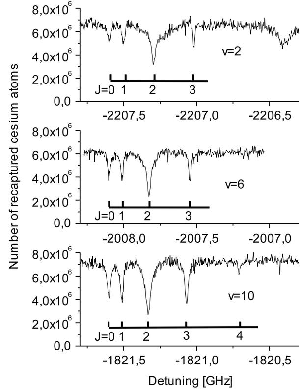
**Fig. 4** Photoassociation trap loss spectra as a function of the photoassociation laser detuning relative to the  $6s\ ^2S_{1/2}(F = 4) \rightarrow 6p\ ^2P_{3/2}(F' = 5)$  asymptote for  $v=2, 6$  and  $10$  in the  $0_g^-$  outer well. Rotational progressions are observed for each vibrational level up to  $J=3$ . For  $v = 10$  also a weak  $J=4$  transition is observed. The resonance at  $-2208$  GHz detuning in the upper panel is attributed to another electronic state.
