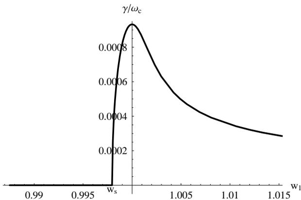
FIG. 2: Decay rate  $\gamma/\omega_c$  of the unstable mode as a function of  $w_1 = \omega_1/\omega_c$  for a fixed value of  $\omega_c$ . The decay rate does not diverge at  $w_1 = 1$  even though we have assumed the waveguide is made of a perfectly conducting material. At  $w_1 = 1$  we have the maximum value of  $\gamma$ , which depends non-analytically on the coupling constant  $g$  as presented at Eq. (10).
