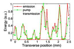
FIG. 4. (Color online) Spatial variation of transmitted energy of the pump beam with fixed input power of  $10 \mu J/pulse$  (dashed curve), and of the total laser energy (solid curve) for a stack of 50 glass slides with a single layer of dye solution in the center.
