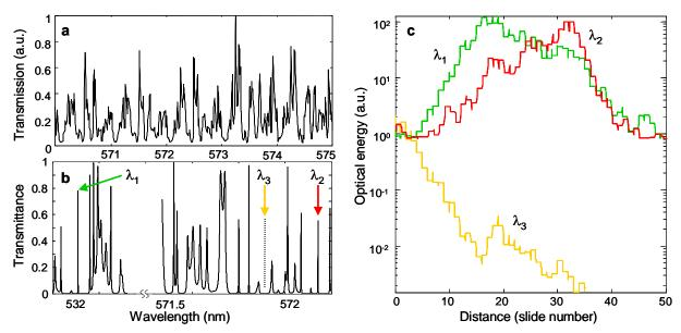
FIG. 3. (Color online) (a) High-resolution experimental spectrum of transmission through a stack of 50 glass slides. (b) Results of a scattering-matrix calculation of the transmittance spectrum for a stack of 50 slabs of random thickness illuminated by a plane wave. (c) Calculated spatial energy distribution of a plane wave incident upon the sample in (b) for the three wavelengths indicated. A stepwise change in energy density occurs at the air/glass interfaces.
