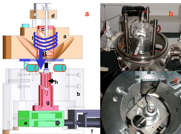
Fig. 2a. Drawing of the STM head: a) top cylinder, b) hollow cylinder, c) magnet, d) magnet slide, e) X-Y coarse positioning, g) piezo tube support, h) piezo tube, f) X-Y motor, l) magnet additional coil. **b** and **c** overview of the entire ESR-STM and detail of the STM tip mounted on the X-Y translation stage
