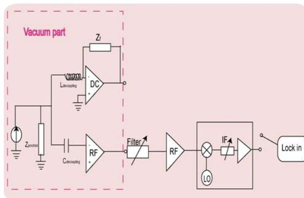
Fig. 1. Overview of the DC/RF recovery circuitry. The STM tunneling junction is considered as a current source with a parallel impedance. The current is split into the RF and DC part. The RF component is amplified close to the junction. Afterwards the signal is feed into a second amplification stage and then to a spectrum analyzer.
