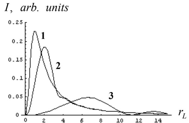
Fig. 3. Radial distribution of OTR intensity on the lens surface for different parameter  $R$  values (Curve 1 -  $R = 10/2\pi$ ; 2 -  $R = 1/2\pi$ ; 3 -  $R = 0.1/2\pi$ ).
