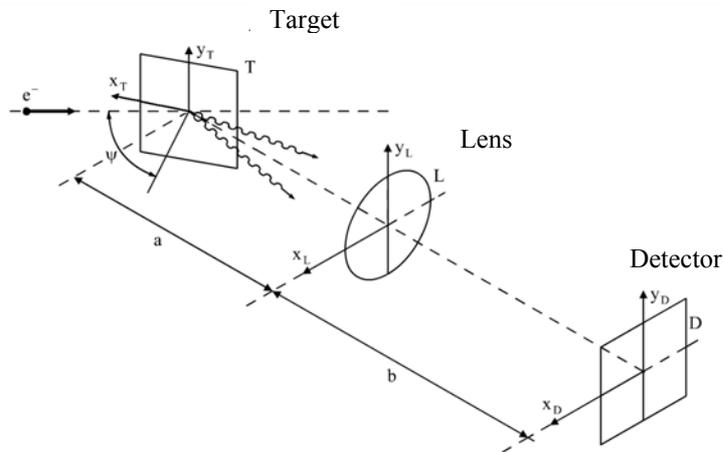
Fig. 1. Optical system scheme of OTR beam size monitor.
