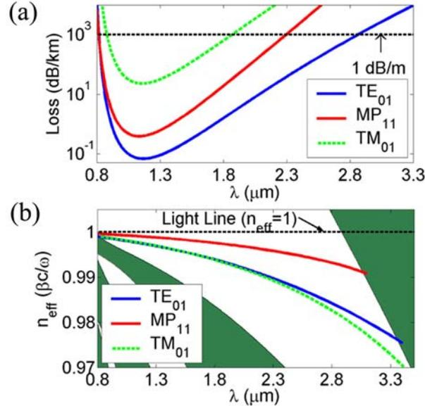
Fig. 2. In (a) and (b), we respectively give the loss and dispersion of the  $TE_{01}$ ,  $TM_{01}$ , and  $MP_{11}$  mode of a Bragg fiber with four cladding pairs, where we use  $n_s=1.45$ ,  $L_s=0.37\mu\text{m}$ ,  $n_l=1.0$ ,  $L_l=4.10\mu\text{m}$ . The shaded area in (b) indicates the existence of propagating modes in the fiber cladding.
