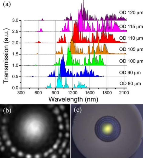
Fig. 4. (a) The experimental transmission spectra of the OD120, 115, 110, 105, 100, 90, and 80  $\mu\text{m}$  samples. (b) The experimental mode profile in the OD90 sample at a wavelength of 1060 nm. (c) The image of the output facet of the OD105 sample with white light input.
