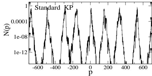
FIG. 4: Floquet states for the standard QKP, for  $K = 3.4$ ,  $\hbar = 1$ . As expected, all the states are exponentially localized, giving the characteristic triangular shape of  $N(p)$  when plotted on a logarithmic scale. They all have approximately similar localization lengths.
